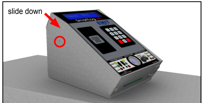
Figure 14. Sliding the SmartLog V5™ into the bracket and securing it into place with the 4-40 screw
